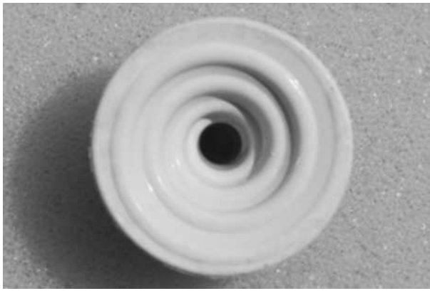
Fig. 1 Design of tested aluminium oxide PIM part
