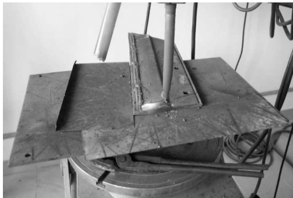
Fig. 2 New surface created by means of overlaying – Automatic welding machine ESAB LAF 635 DC
