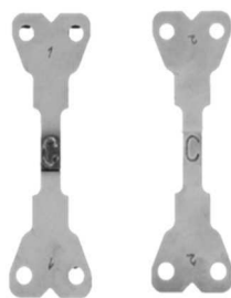
Fig. 3 Specimens welded by laser beam (left) and electron beam (right)
