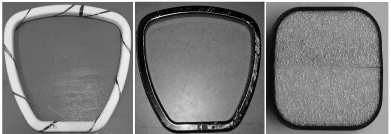
Fig. 9 Laboratory samples from winding process with data of numerical model
