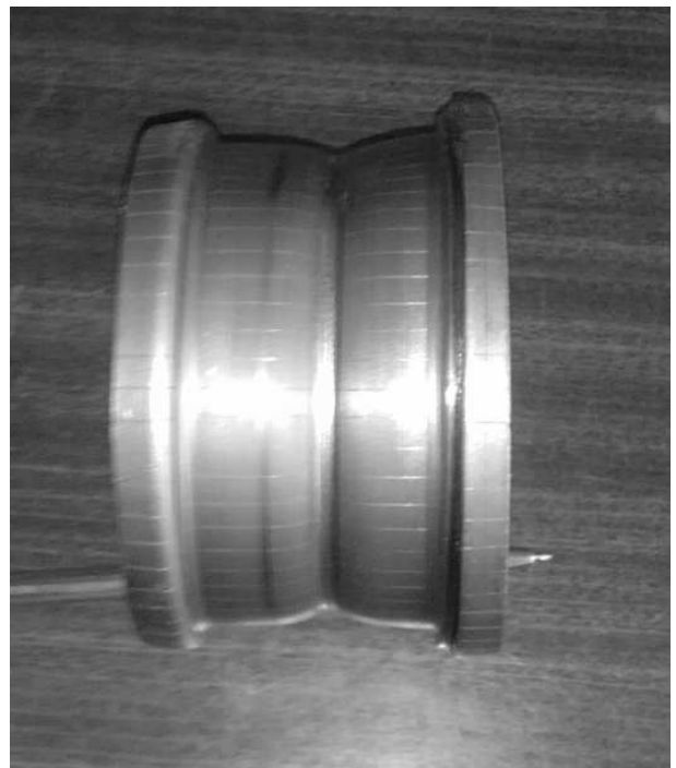
Fig. 3 Attachments for applying technological corrugations (a), and a semi-finished product with a corrugation
