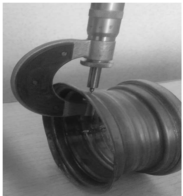
Fig. 4 The measurement of the thickness of the metal in the curved areas of the profile of the semi-finished product
