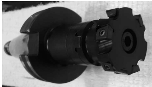
Fig. 3 New cutting tool for machining the T-groove detail [1]
