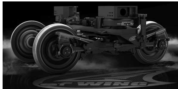
Fig. 2 The bogie of the passenger wagon "efWING" with the use of an elastically dissipative carrier element
