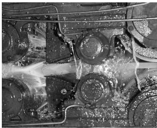
Fig. 1 Rapid quenching of Armox steel by water [2]
