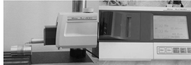
Fig. 2 Measuring experimental parts using Mitutoyo SJ-400
