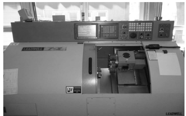
Fig. 1 CNC lathe Leadwell T-5
