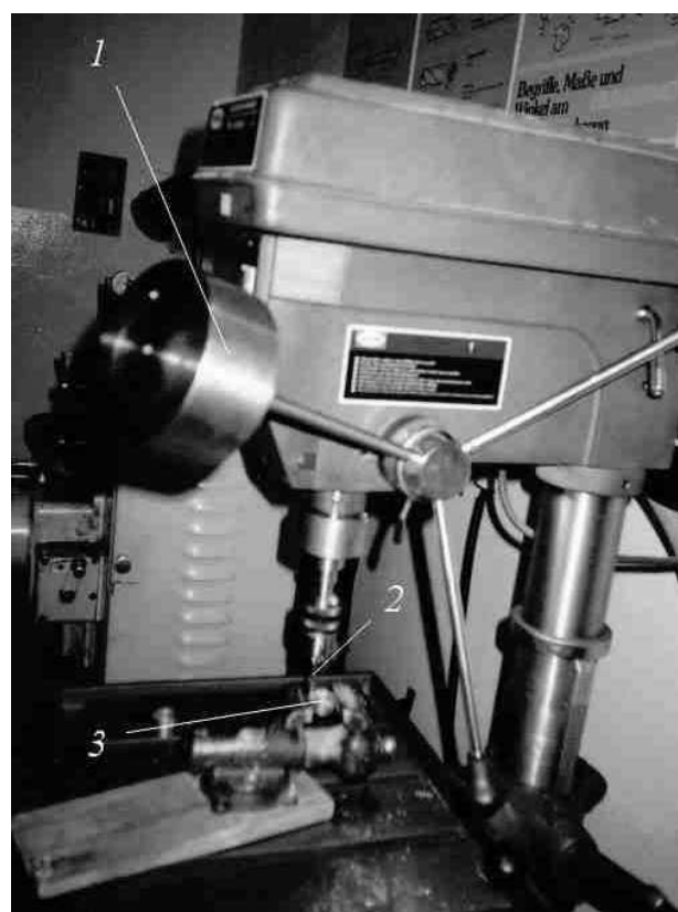
Fig. 2 Drilling with constant axis force with table drill. a – load scheme, b – actual drilling 1 - weight, 2 - drill, 3 - workpiece
