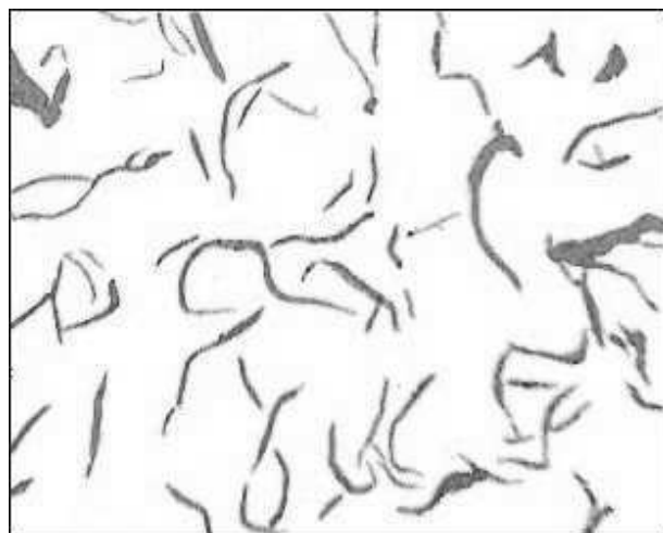
Fig. 2 Microstructure of grey cast iron, 100x zoomed
