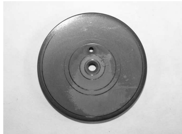
Fig. 1 Drawing of the experimental sample with said manufacturing dimensions (left) and the appearance of the sample after the measurement of the coefficient of friction using the "Pin on disc" (right)
