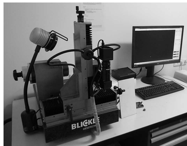
Fig. 3 Optical microscope Multicheck PC 500
