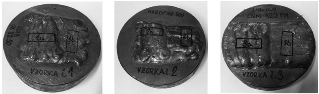
Fig. 6 Samples No. 1, 2, 3 - weld deposits (a-double layer, b- single layer)
