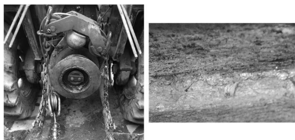
Fig. 1 Winding drum with directional pulley and detail groove pulley after wearing
