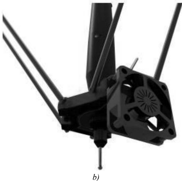
Fig. 5 Replaceable print heads and their applications to delta, laser (a.), milling spindles (b.) [8]
