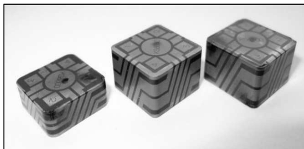
Fig. 3 Ceramics inserts with applied resistance layer
