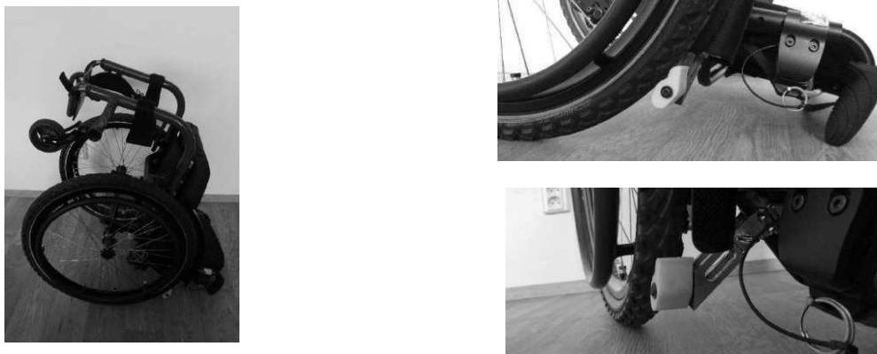
Fig. 8 Positioning of the assistance brake for possible damage during use or fall [1]
