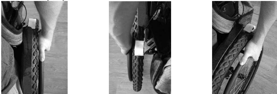
Fig. 7 Position of the assistance brake in terms of possible injury [1]
