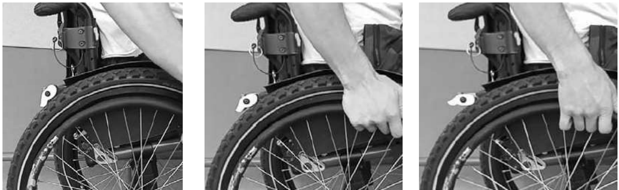
Fig. 10 Braking segment movement during braking [1]
