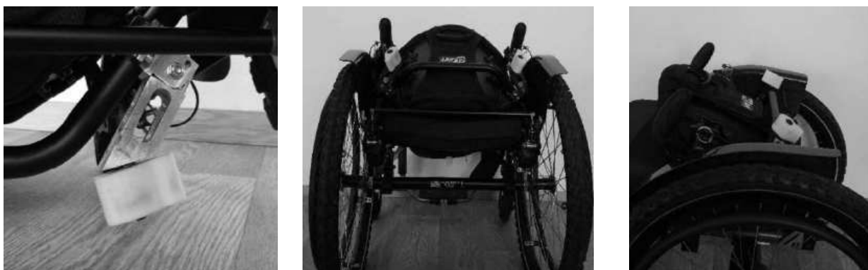
Fig. 9 Fold ability of the wheelchair with assistance brakes during transport [1]
