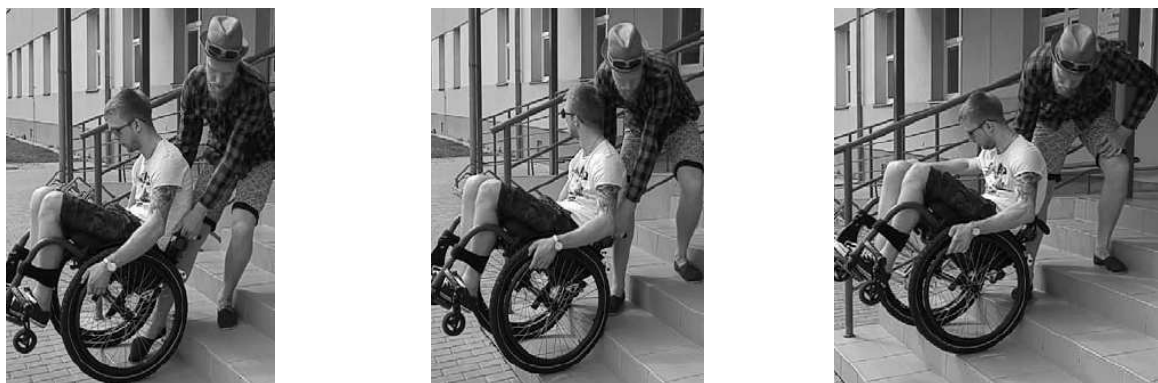
Fig. 11 Exit the wheelchair using the assistance brake [1]
