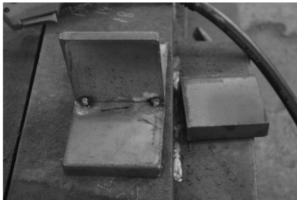
Fig. 7 The T-joint with single V groove before welding
