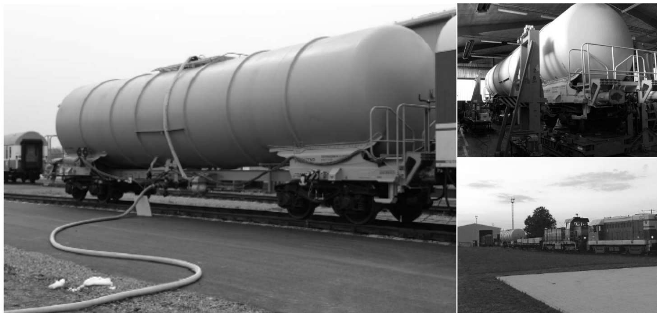
Fig. 9 Static, fatigue and ride tests of tank wagon prototype
