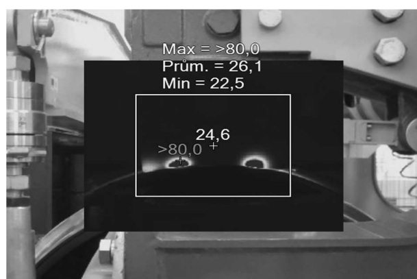
Fig. 7 Temperatures detected by thermal camera FLUKE at the beginning of braking
