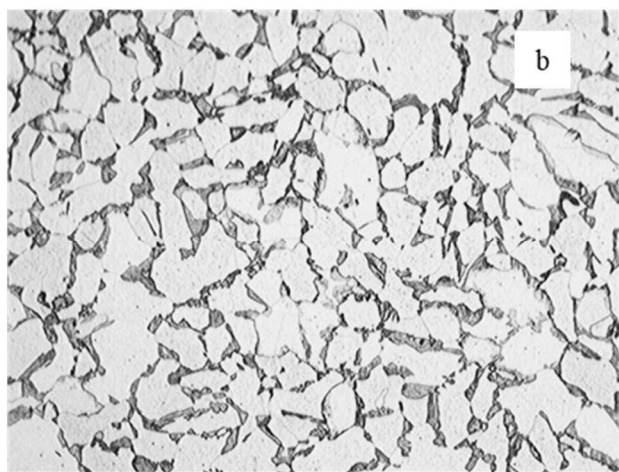
Fig. 5 Microstructure of the knife material a) the transition region from the body to the cutting part of knife b) microstructure of the body knife
