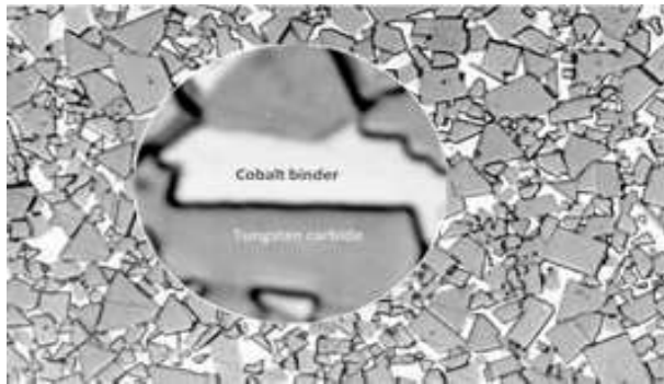
Fig. 1 Structure of a cemented carbide and the formation of bonds between the hard carbide and the binder metal. The second micrograph illustrates a new trend in cemented carbides, where vanadium carbide serves to impede the propagation of cracks [5].
