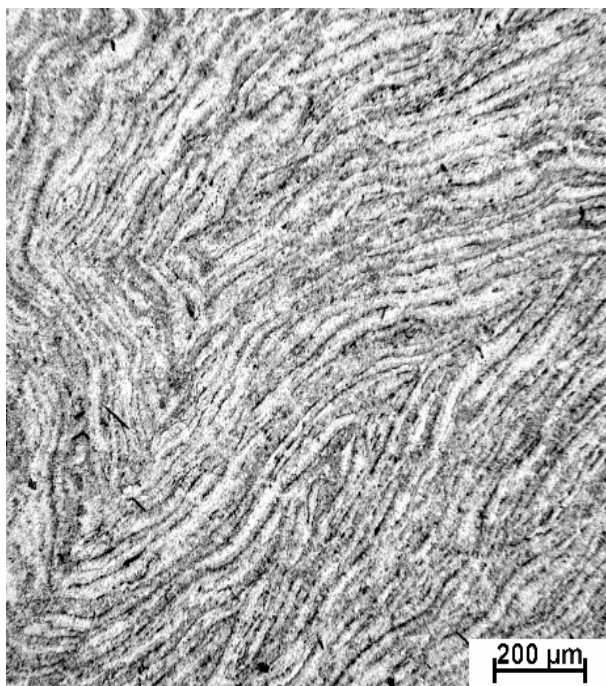
Fig. 7 Microstructure of bulk AlFe7Mm4 alloy, B1 (LM)
