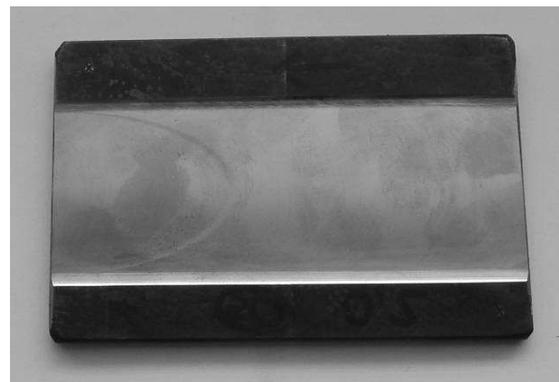
Fig. 3 Sample photo after hard milling, sample width 70 mm
