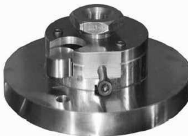
Fig. 7 Special fixture for clamping tested samples [4]
