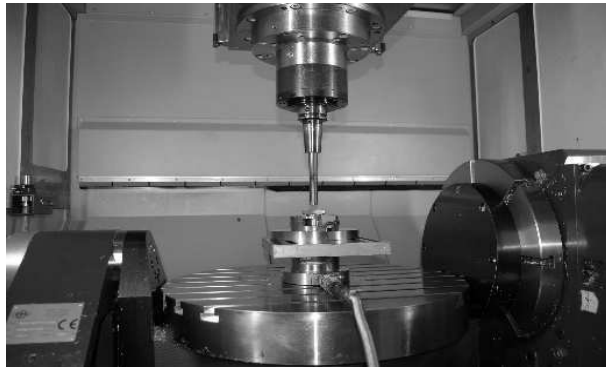
Fig. 4 Scheme of measurements using piezoelectric dynamometer Kistler 9272 placed on 5-axis CNC machining centre MCV 1210
