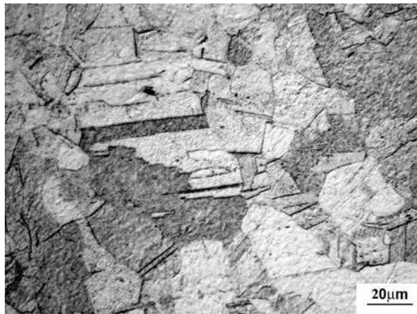
Fig.8 Microstructure of 5h 1938 (CuZn8), cross section (left) and longitudinal section (right)
