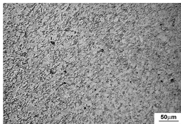
Fig.6 Microstructure of 2h 1923 (Zn), cross section (left) and longitudinal section (right)
