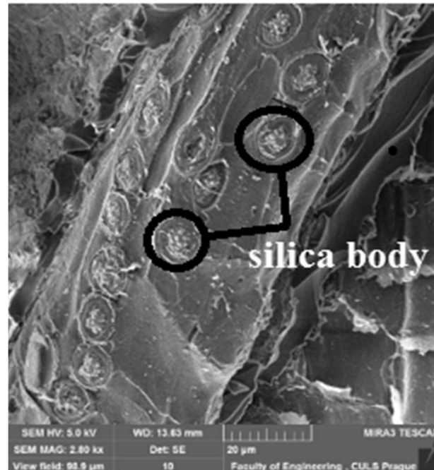
Fig. 8 Structure of EFB fiber surface
