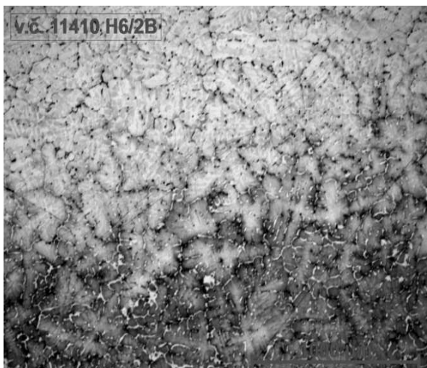
Fig. 10 Fuzzy boundary between defect and surrounding structure after etching
