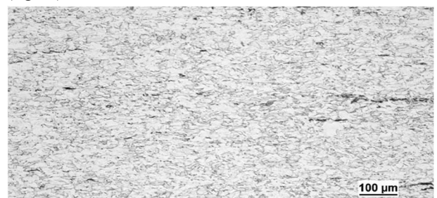
Fig. 1 Structure of steel 1.4571 (316Ti) after cold rolling
