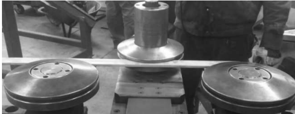
Fig. 2 Material inserted between rollers prepared for bending
