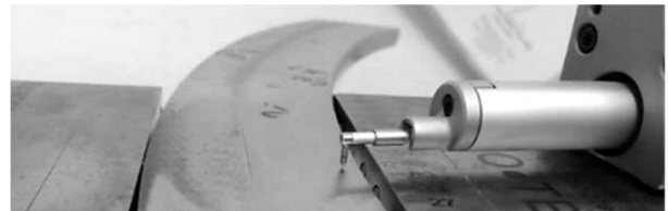
Fig. 6 Process of roughness measurement
