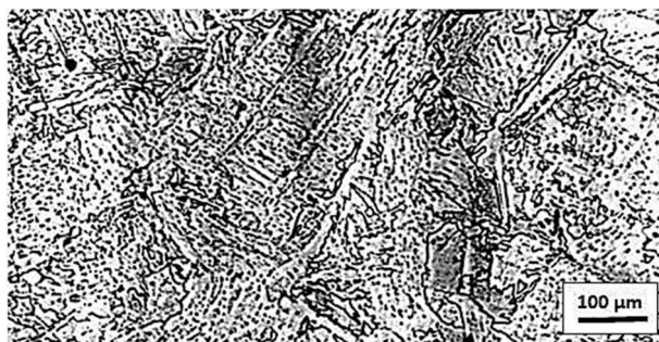
Fig. 10 15 111 steel degraded structure character, upper bainite
