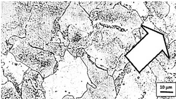
Fig. 5 Degradation structure character of the 15 128 steel after 198.217 hours
