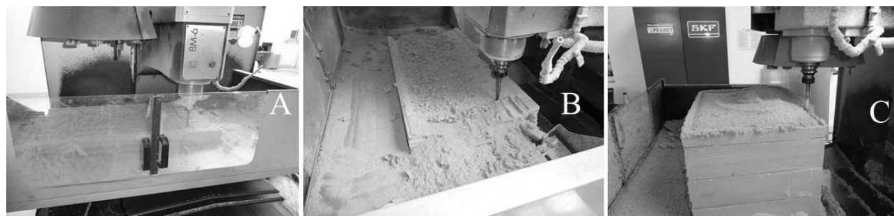
Fig. 1 Measurement of milling: A: MDF, B: detail view on MDF milling, C: Polystyrene
