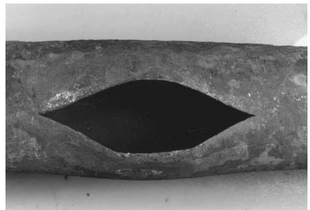
Fig. 2 Surface buckling and tube rupture
