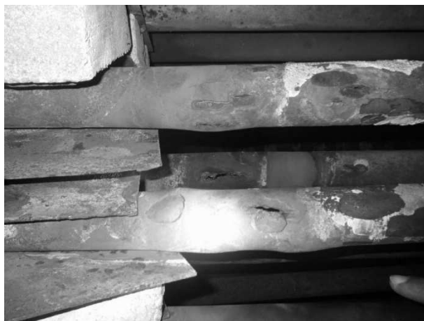
Fig. 1 Tube damage by local creep deformation and macro-crack development
