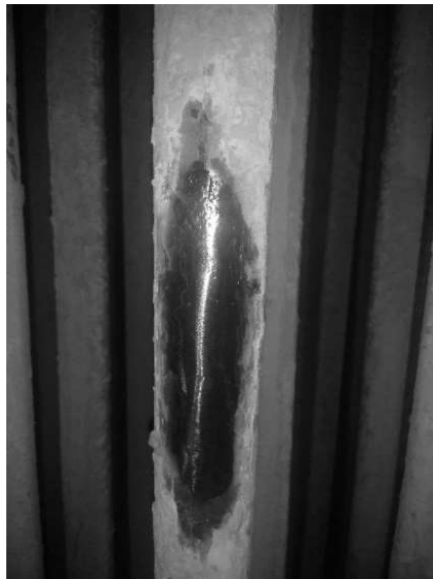
Fig. 4 Ground place for UT inspection, surface detail
