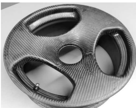
Fig. 4 Carbon wheel disc after demoulding (left) and finishing operations (right)
