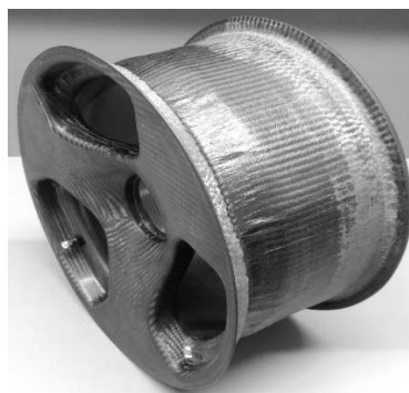
Fig. 4 Carbon wheel disc after demoulding (left) and finishing operations (right)
