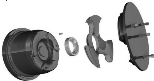
Fig. 2 Mold assembly with aluminium insert (yellow) and honeycomb 3D printed core (green)
