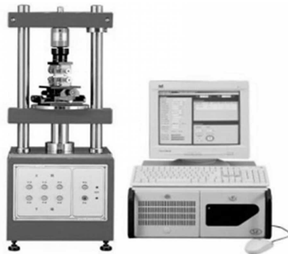
Fig. 4 Structure of the inserting force testing machine
