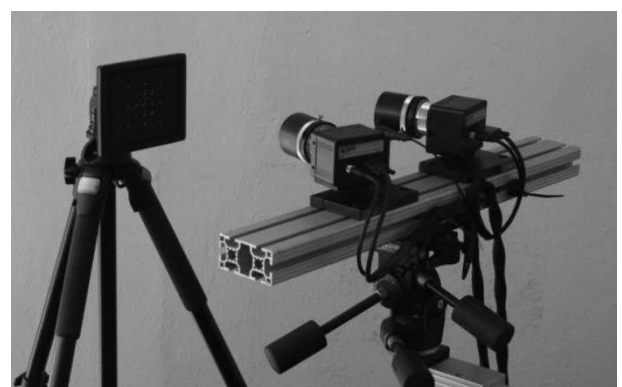
Fig. 3 Calibration panel (GOM MV 90x72 mm 2 ) to carry out calibration of the cameras
