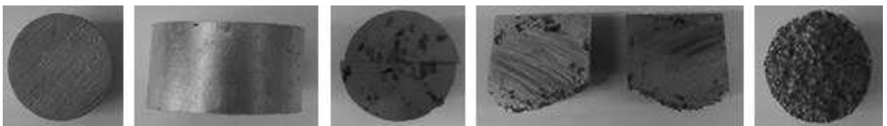
Fig. 5 Sample of pure aluminium for "foaming" (left) and the macro structure of pure aluminium cellular system samples (right)
