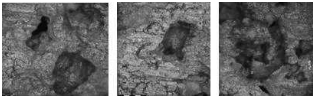
Fig. 8 Porosity of a cross-section sample of porous aluminium AlSi12 alloy, monitored by the Olympus DSX 500 microscope (enlargement 5x)
