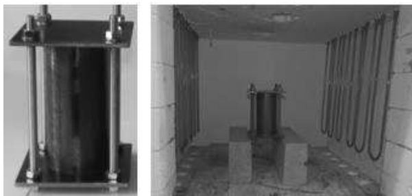
Fig. 4 Preparation jig and furnace for the production of porous aluminium systems
