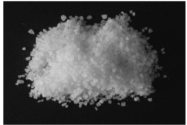
Fig. 3 Sodium chloride used for the production of porous aluminium
