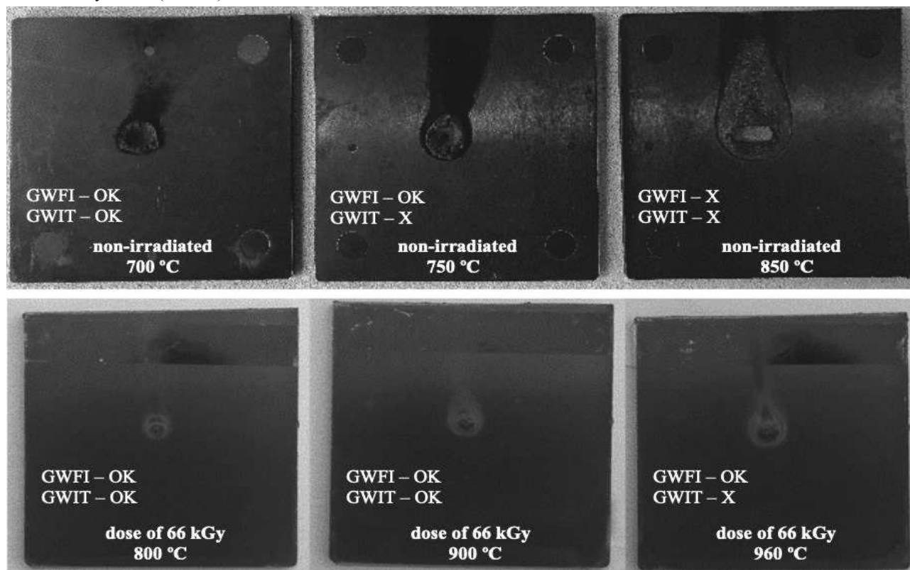
Fig. 5 Test specimens (material PA 7T – 56 % GF) after testing
