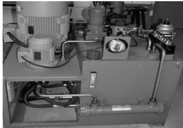
Fig. 7 Experimental equipment of hydrostatic lubrication system for 80 mps high-speed roll grinding head
