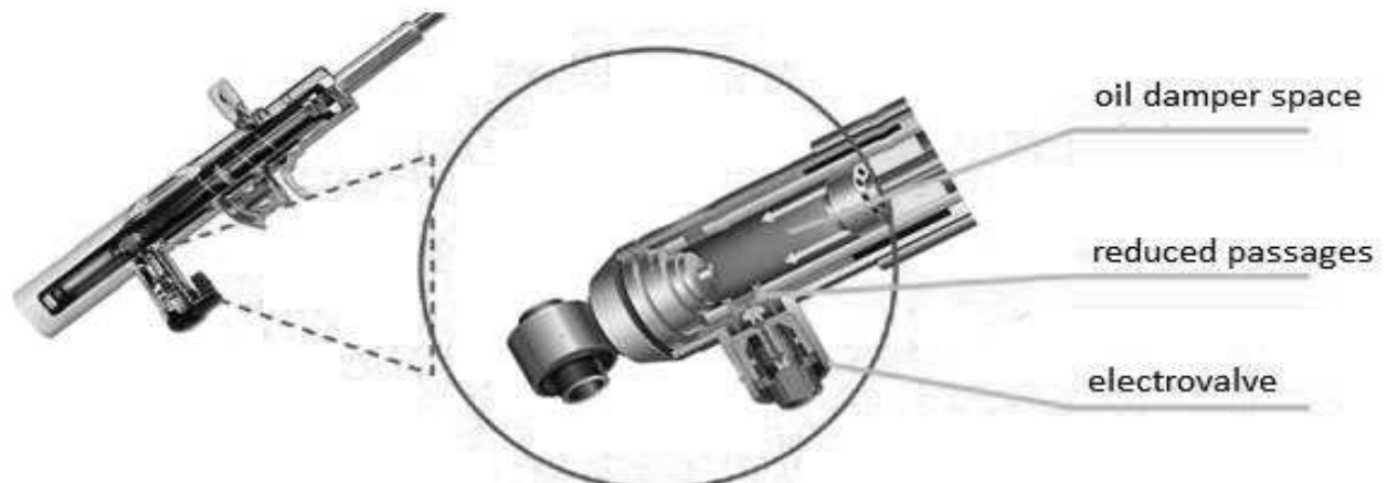
Fig. 5 Diagram of location and principle of the variable damping electrovalve [3]
