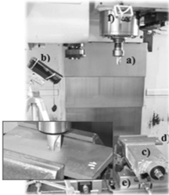
Fig. 8 Experiment procedure a) the milling machine b) the infrared camera MobIR M8, c) the vice d) the machined sample e) dynamometer KISTLER 9255 A, f) the camera GoPro
