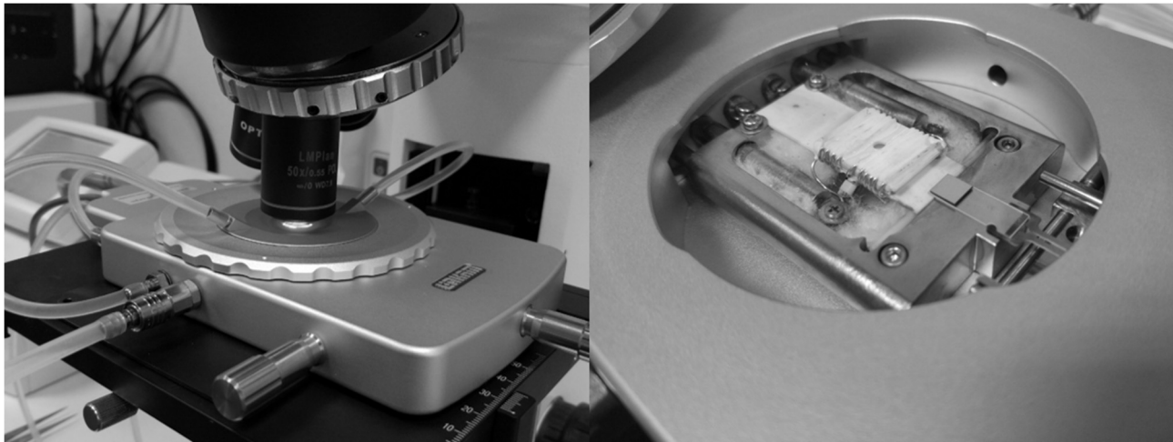
Fig. 1 The chamber during heating to higher temperatures (left), a view inside the chamber with a specimen on a ceramic glass (right) [4]
