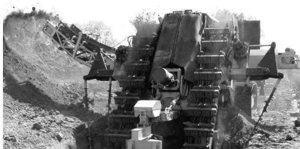
Fig. 6 MV-T-2M pipeline opening machinery with the actuator equipped with impulse soil unloading intensifier
