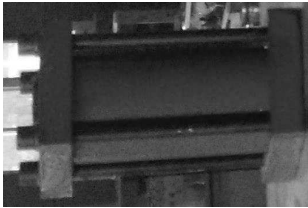
Fig. 26 Hydraulic cylinder loaded on test bench
