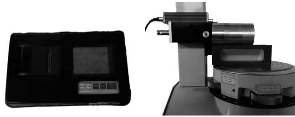
Fig. 2 Portable Surface Roughness Tester
