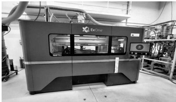
Fig. 4 Additive device ExOne 160L Pro working on the technological principle of Binder Jetting
