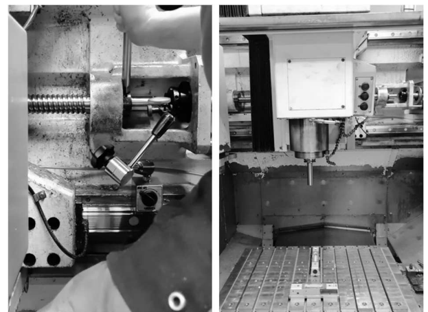
Fig. 12 Ball screw preload adjustment (right) and machine levelling check with spirit levels (right)
