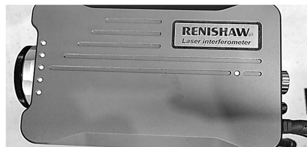
Fig. 7 Diodes on the laser head indicating signal strength
