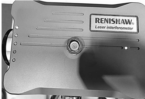
Fig. 2 Alignment of the laser head using a circular level
