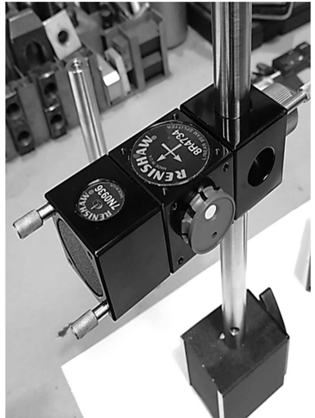
Fig. 4 Interferometer mounted on the machine table with a target
