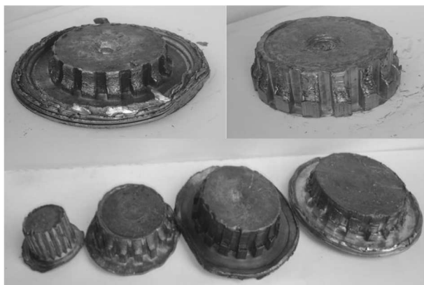
Fig. 18 Formed gears by rotary forging process
