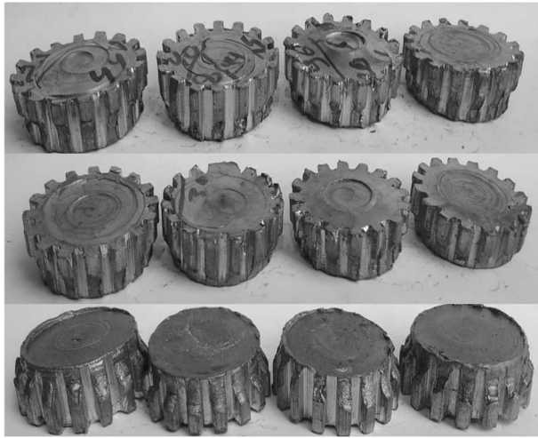
Fig. 22 Successful formed gears at different parameters
