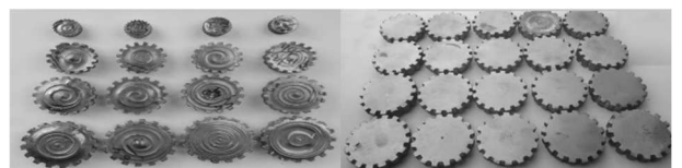
Fig. 20 Successful formed gears at different parameters
