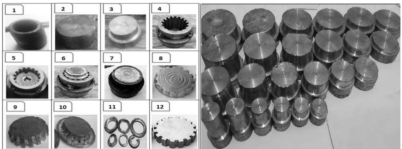
Fig. 8 The blanks used in rotary forging process and experiment preparation steps
