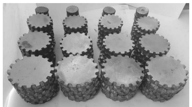
Fig. 21 Successful formed gears at different parameters
