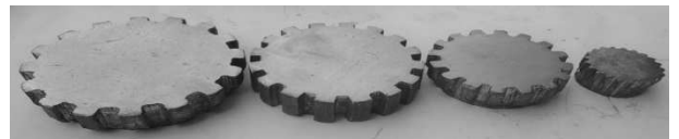
Fig. 19 Successful formed gears by rotary forging process
