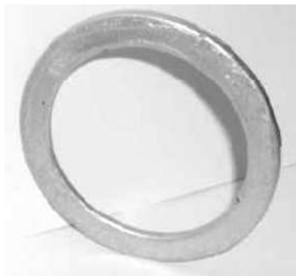
Fig. 3 Carrier with an aluminium layer formed [17]
