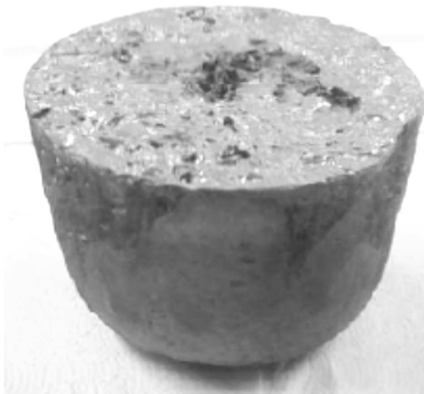
Fig. 6 Casting of sedimenting refining bath
