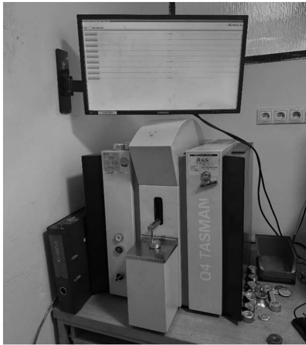
Fig. 3 Digital optical emission spectrometer Q4 TASMAR with a CCD detector
