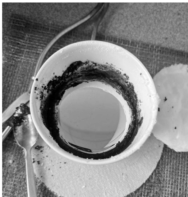
Fig. 2 Sn-P alloy after melting process
