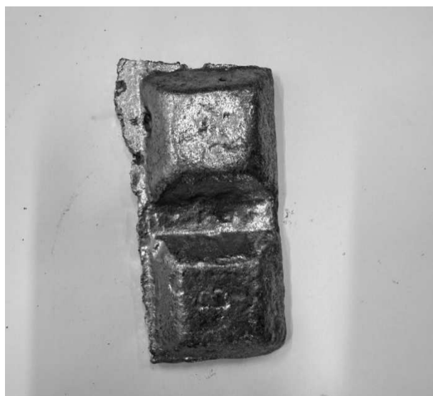
Fig. 4 SnP2 alloy in waffle shaped ingots
