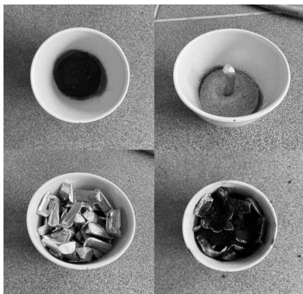
Fig. 1 Preparation of Sn-P alloy batch
