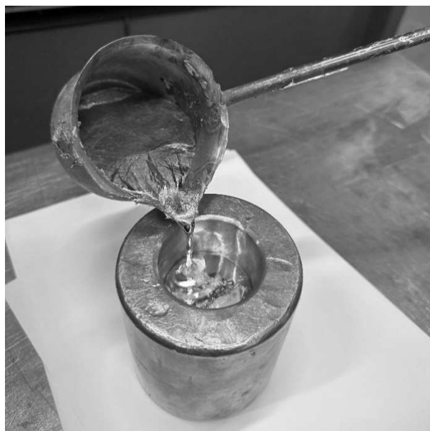
Fig. 5 Brass mold for samples of melted solder alloy SAC305
