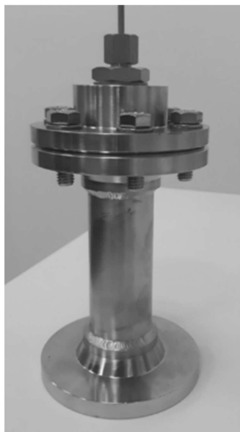
Fig. 1 Test vessel for molten salt corrosion experiment: as-received condition and dimensioned drawing
