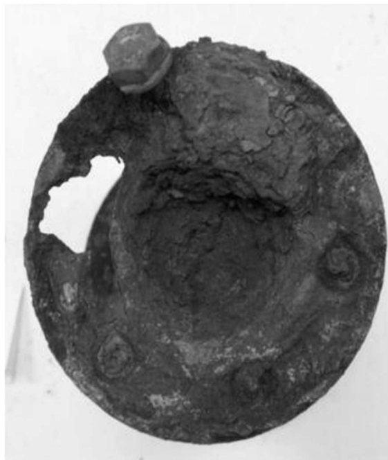
Fig. 3 Detail of corrosion damage of Test vessels exposed to FLiNaK salt (specimen C on the left, specimen D on the right)
